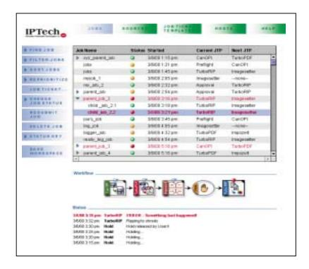
nAct's Workflow Engine maintains a dynamic internal database, which presents an overview of the entire production workflow, with current disposition and detailed status of every job, via nAct's web browser-based Job Monitoring and Control GUI.
